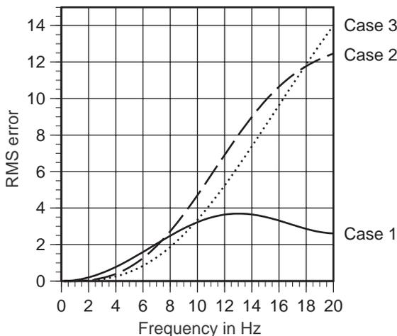
Figure 8: RMS error for Kalman predictors, 50 ms interval
