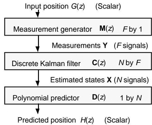
Figure 5: Kalman filter transfer function dataflow
