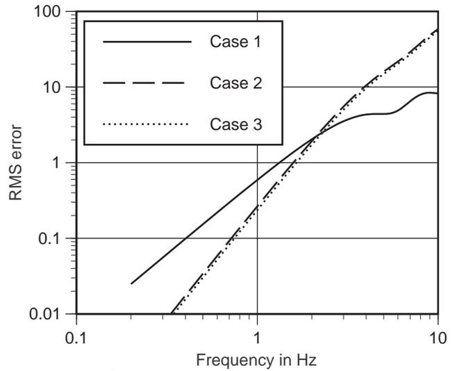
Figure 9: RMS error for Kalman predictors, 200 ms interval
