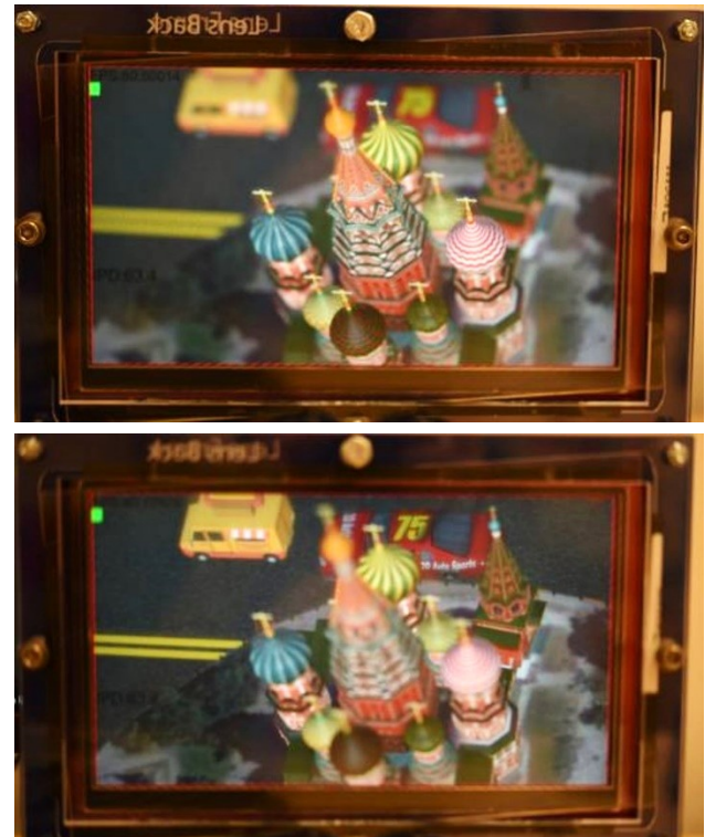
Figure 8. Captured images from system 1 prototype. Top: Camera focused at near distance. Bottom: Camera focused at far distance. Content: Stockcar racecar (Unity asset store license) and St. Basil's Cathedral (3D Warehouse license)
