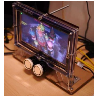
Figure 6. 72 PPI light-field display prototype with stereo cameras for eye position tracking.
