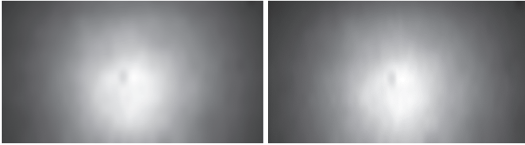
Fig. 8. Beam profile using scanning grating and photodiode (left) and using vertical TWINS (right).
